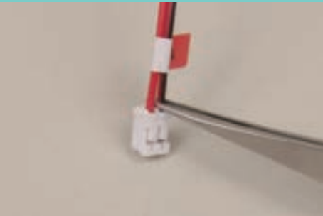
Hold its base with tweezers as shown when inserting the connector. Align the connector with the socket as it is and plug it in, while taking care not to grip it too tightly as it could damage the cable.
