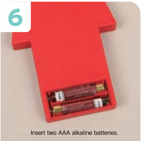
Get ready two AAA alkaline batteries, and insert them into the Remote Control Case. The springs are for the negative poles (-).
