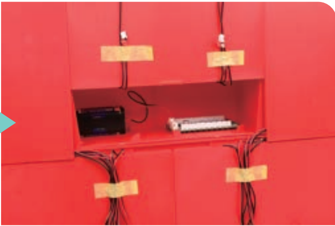
Pull the cables at the opening at the back of the doghouse outwards, and insert the Circuit Board Case from step 50 as shown.
